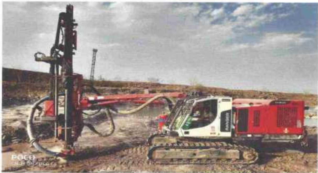
Typical View of Drill with Dust Extractor system equipped with water injection system
